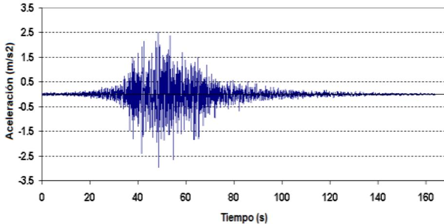
Figure 3. Moquegua earthquake acceleration record on 06/23/2003.
