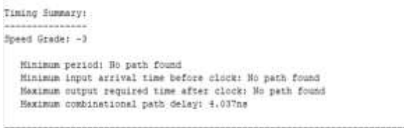
Fig 20: synthesis report for Delay in proposed 15:4 counter
