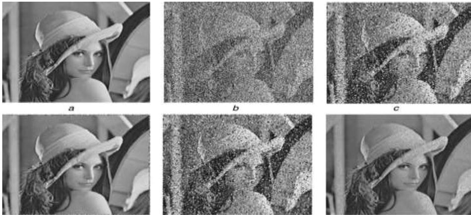
Figure 9. Visual performance of MF-DC. (a) original image, (b) noisy image, (c) SMF [11], (d) DMF [12], (e) AMF [13], (f) proposed MF-DC.
