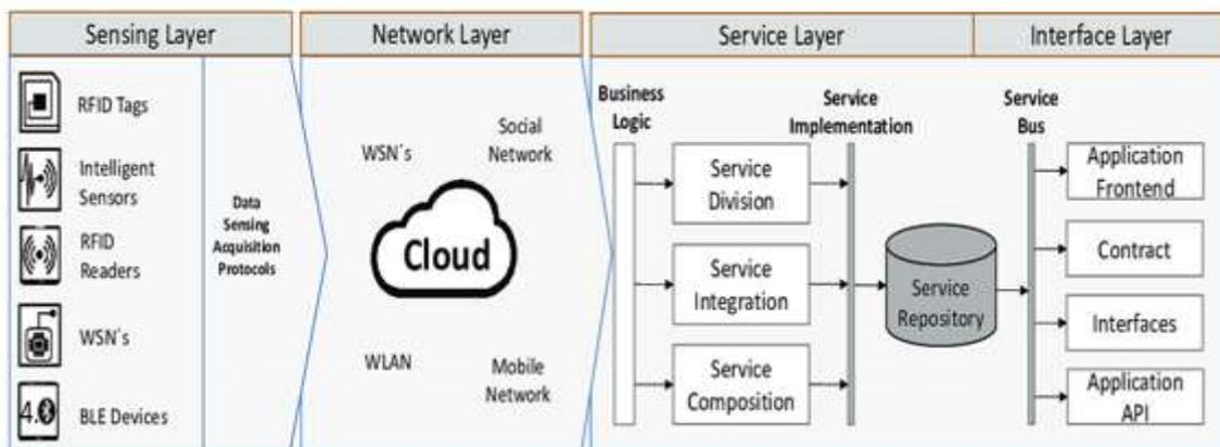
**Fig. 4: IOT Based Service Oriented Architecture**
