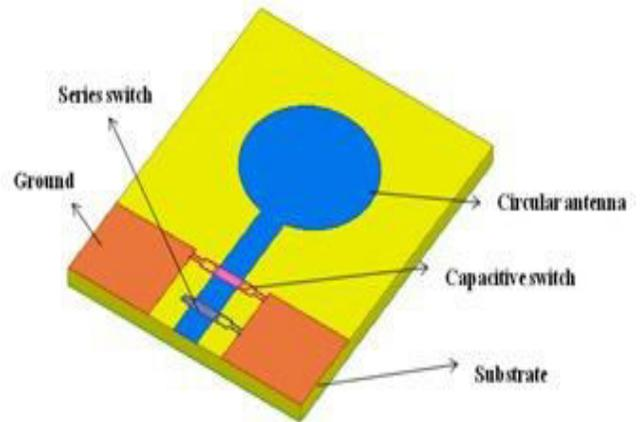
**Fig.2:** Schematic representation of the proposed Hybrid switch
