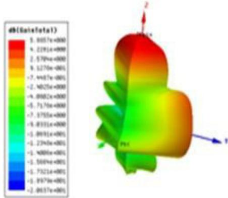
**Fig.8:** Gain of the Hybrid RF-MEMS switch
