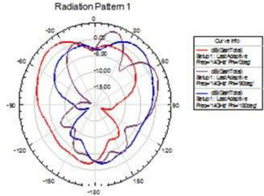
**Fig.10:** Simulation of Radiation pattern of Hybrid switch
