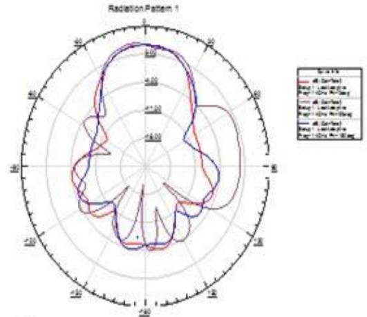
**Fig.6:** Radiation pattern of the proposed antenna
