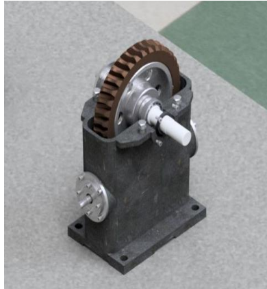
Figure 3: Visualization of the project "Worm gearbox", made by a third year student at the classes on applied mechanics in Autodesk Inventor.
