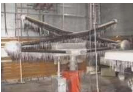
Figure 1 Vertical break disconnectors with ice loading under test
