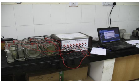
Fig. 2 Rapid Chloride Permeability Apparatus
