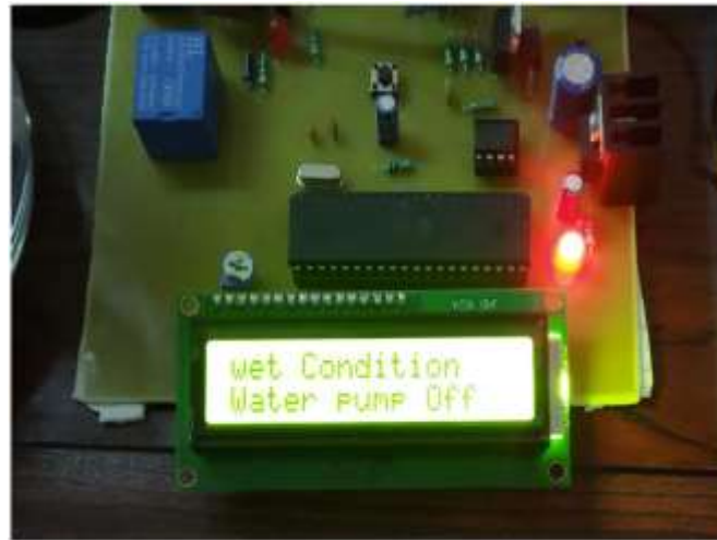
Figure.9. Operation of the Hardware setup showing soil wet condition and status of the pump in OFF condition
