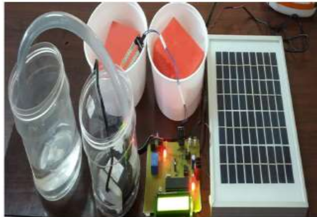
Figure.6. Operation of the Hardware setup of the proposed irrigation system using solar power under soil dry condition
