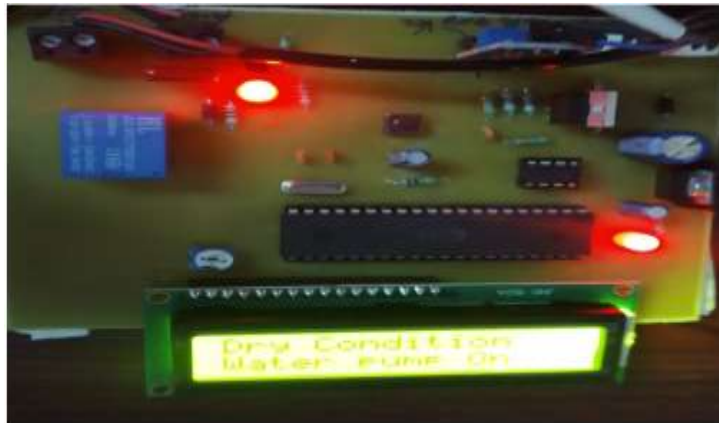
Figure.7. Operation of the Hardware setup showing soil dry condition and status of the pump in ON condition
