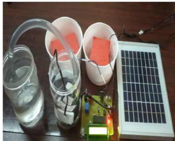
Figure.8. Operation of the Hardware setup of the proposed irrigation system using solar power under soil wet condition
