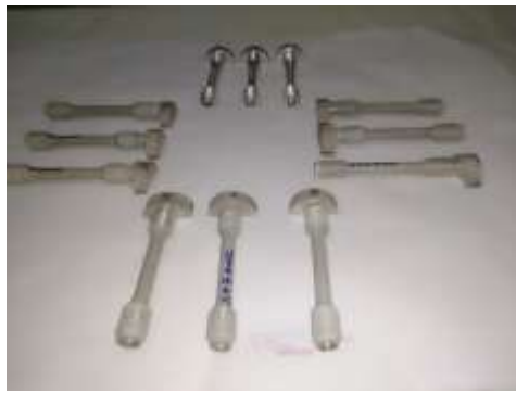
Fig. 8 (a) Native samples (b) Deep cryogenic-treated samples
