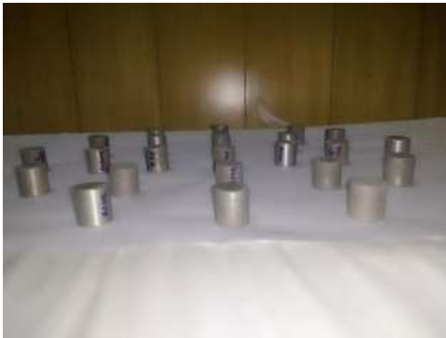
Fig. 2 Sectioned samples for the metallographic studies
