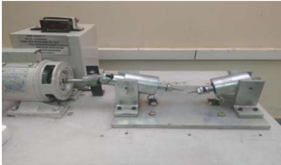
Fig. 10 fatigue test apparatus for the native and DCT-treated samples
