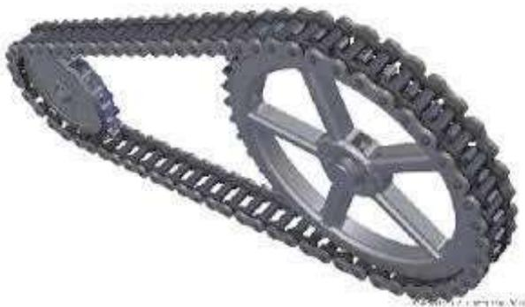
Sprocket wheels and chain are the kind of mechanism which are used for transferring the rotary motion to the DC motor from the rack and pinion.
